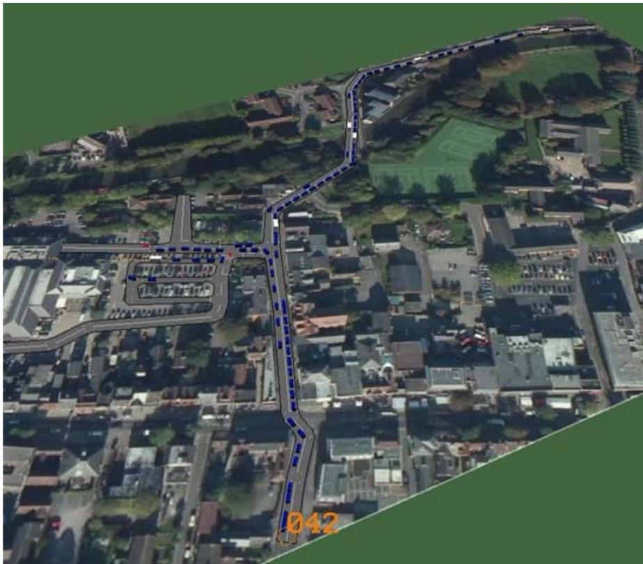
Figure 3.5 PARAMICS Traffic Model Visualisation for Saturday 11.39 am with the MSCP, showing the queue that has built up on Kings road. The number 42 indicates the additional 42 cars in the Kings road queue which are not shown on the display.
