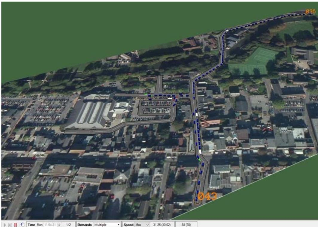
Figure 3.6 PARAMICS Traffic Model Visualisation for Saturday 11.54 am with the MSCP, showing the queue that has also built up on Lower Kings road stretches back to the station with the additional 36 cars beyond the station not shown on the display.
