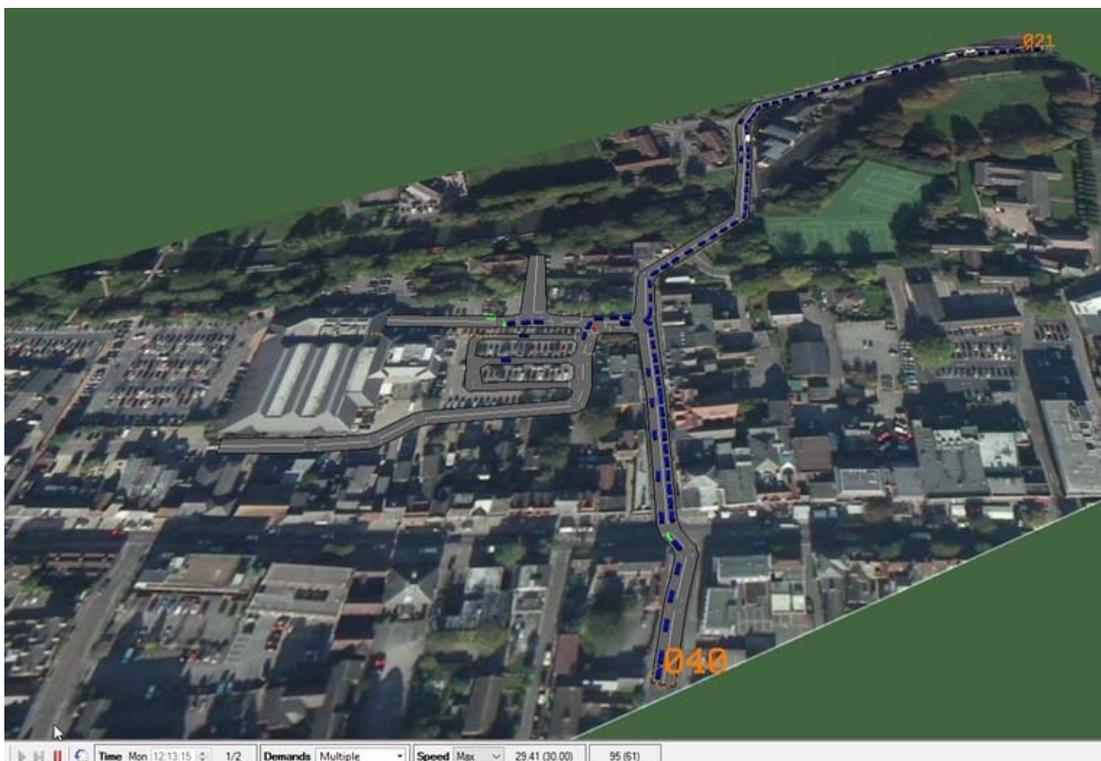
Figure 3.7 PARAMICS Traffic Model Visualisation for Saturday 12.13 am with the MSCP, showing that the Lower Kings road queue has 21 cars beyond the station and 40 cars up the Kings road hill not shown on the display.
